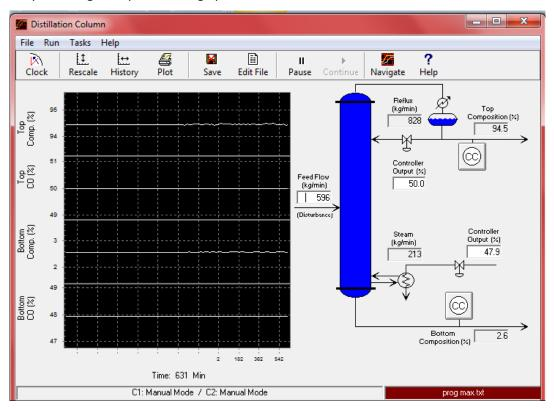
I choose to perturb the system by changing the value of the disturbance from 595.95 kg/min to 700 kg/min (arbitrarily chosen) with a ramp rate set by default 0.10 kg / min / min.
