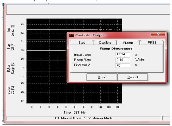
Made the variation, the variables can be represented as a function of time. Following the "limited" ramp, CO moves to new steady state.
