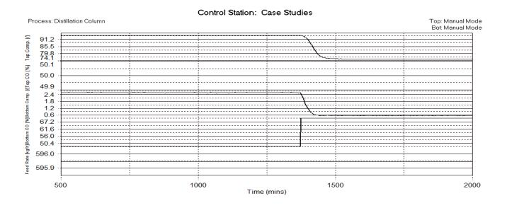
In the second case, by varying the CO to limited ramp, the system moves to a new steady state value more slowly and the compositions of both top and bottom decrease.
