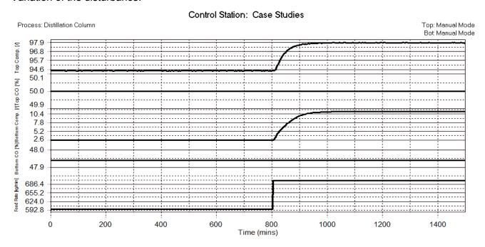
In the first case the variation of the disturbance step involves a variation of the system towards a new equilibrium state. In fact, in the distillation column there will a new value of the composition for both, top and bottom. In particular, the composition increases. Moreover, the values moves in a new steady state asymptotically.
