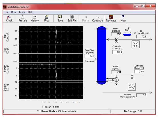
In the following graph, all the variables are represented as a function of time. The behaviour of the variables changed, moving for a new steady state after the disturbance.
