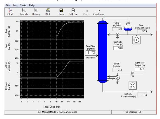
The disturbance has a variation on "limited" ramp. The system, moreover, moves to a new steady state.
