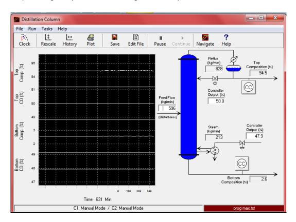
I choose to perturb the system changing the control output to the final value from 47.94% to 70% (arbitrarily chosen).
