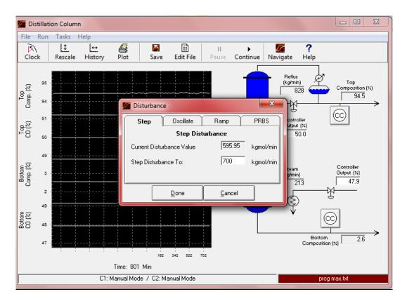
I choose to perturb the system changing the value of the disturbance from 595.95 kg/min to 700 kg/min (arbitrarily chosen).
