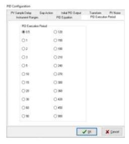
By setting the PID Execution Period as low as possible, we ensure that the PID responds with a high speed and therefore is faster in carrying out its action.
