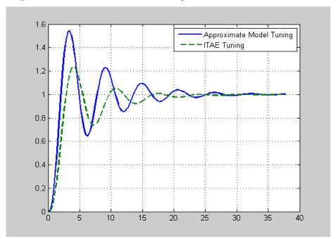
Then, the same **PID** controller is subjected to an ITAE *tuning* procedure and the dynamic system controlled by it at closed loop is again subjected to a *step* response in the *set point* (see the **dynamic response** with dashed curve in fig.).
