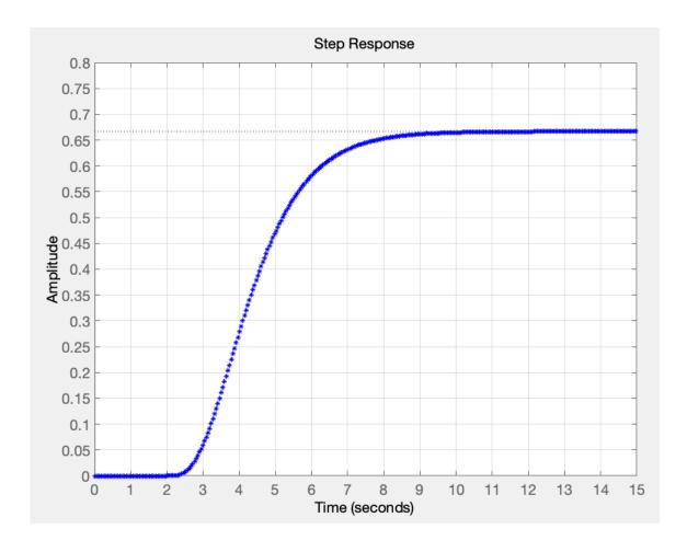
Approximate the **open loop transfer function**, whose step response is in the figure above, with a FOPDT transfer function.
