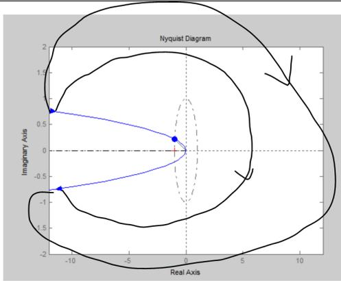
$2\pi$  clockwise at infinity from  $\omega = 0^-$  to  $\omega = 0^+$
